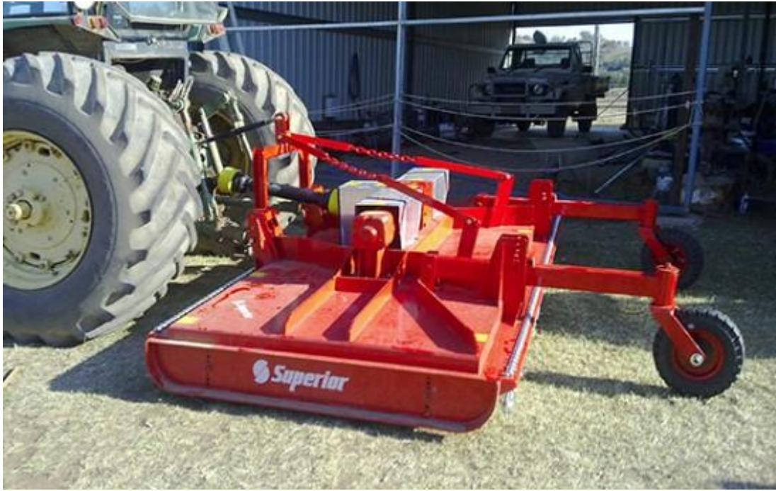
Figure 1 Superior 8 foot pasture topper similar to the one described
