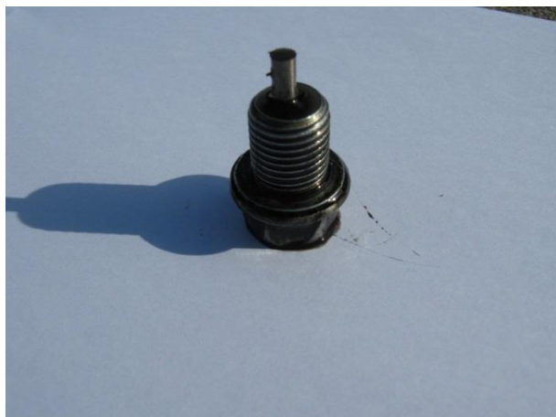
Figure 2 XT600 ~80,000 km magnetic sump plug during oil change showing almost no ferrous metal
