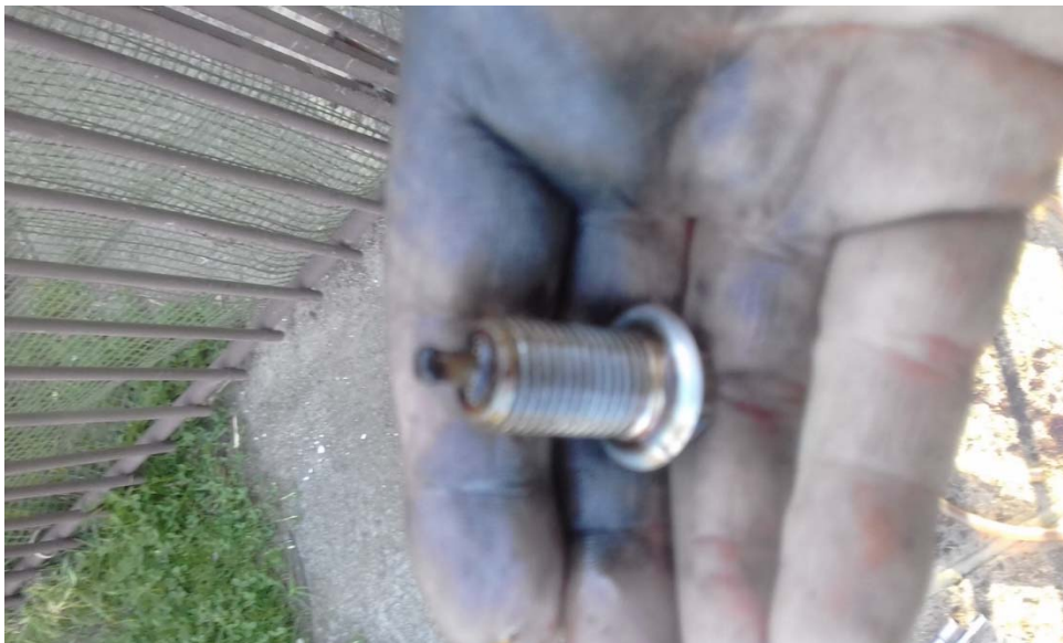
Figure 2 Engine oil sump plug with magnet. Note the small amount of ferrous metal on the magnet.
